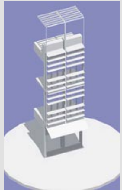
Horizontal and vertical shading devices protect interior spaces from hot, summer sun, thereby greatly reducing cooling loads for the building.
